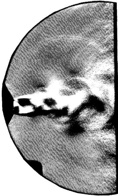
Fig. 6a Schlieren picture showing a supersonic impinging jet undergoing antisymmetric feedback instability; M_j = 1.29 , L = 3.45 in., f = 6.3 kHz.
